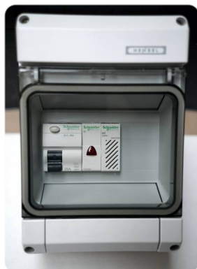
Alarm box (with electric shock protection in the form of a residual current breaker). Additionally equipped with light and sound alarm. in a 6-module casing with IP 65 rating. The box is used in pumping stations as well as in outlet and retention tanks.
